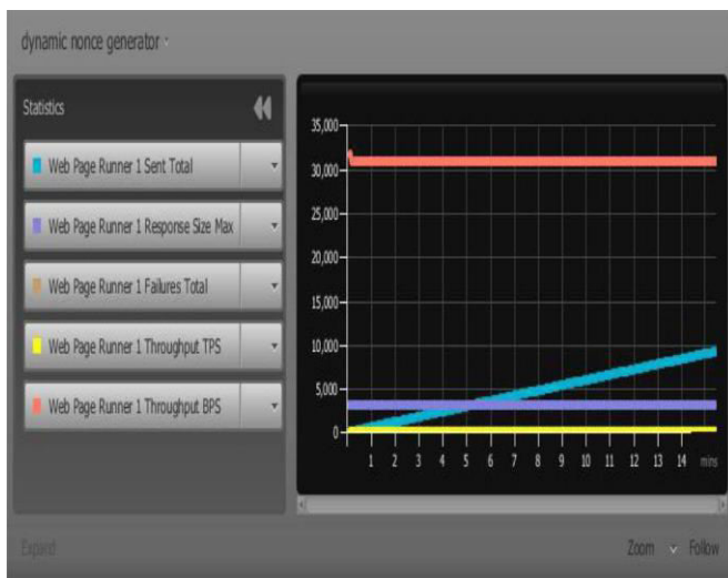
Figure 6.2 The performance results of authentication approach against total request sent, response size, failures, TPS and rate.
